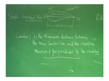
So, if you have commonsense, you can find out what is camber, I need not all these follow this definition. So, is the maximum distance between the mean camber line and the chord line, this is important measured perpendicular to the chord line. This is important, the here which are the chord line is horizontal here.
