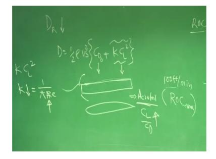
If I want to see the power required is less; that means, a drag required for a given speed should be less and what is the meaning of drag required being less I see drag required if I want to be low then drag is nothing but half rho V square S C D naught plus K C L square.
