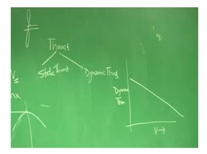
If you are using a propeller driven engine then you know when I talk about thrust may something called static thrust another is called dynamics thrust you can very well understand the very mechanism of thrust developed by the propeller we are not going into any equations or any technical term the propeller develop thrust by pushing the air backward.
