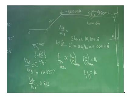
So, I have handled 0 to 1, warm up and take off then climb, this is 2 then I am going for first range which is around 9114 triple 0 feet. So, upto this if I put a 0.3 and 0.4 here this is representing a loiter let us say loiter in that example is for 3 hours, then it goes again comes back again loiter for 30 minutes, and land this is the machine requirement.
