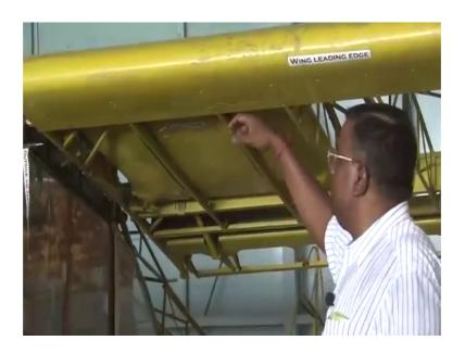
So, design combinational refine people are putting fuel tank inside the wing right; that means it is just not selecting an aerofoil we need to see that when I translate that into a wing I should have enough volume to accommodate this tank.
