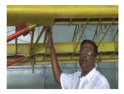
Now, beyond aerofoil and fuel tank if we said these are one this ribs they actually maintain the contour of the wing and the question comes how many of such ribs should be there how many of load bearing member longer on (Refer Time: 17:04) will be there we after all, it will always having a bending load or torsional load how do I distribute those load across the member through this sort of a structure and ensure that they are plenty safe structurally.
