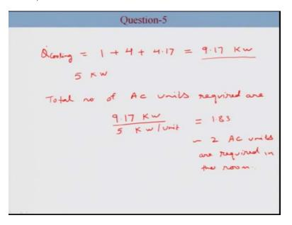
So, total load for air conditioners is 1 because of the light, 4 because of the people and because of the heat gain it is 4.17. So, this sums up to 9.17 kilowatt, so 9.17 kilowatt is to be removed from the room. So, total numbers of AC units required are total cooling load divided by the cooling capacity of one AC or this is equal to 1.83 and so approximately 2 AC units are required in the room.
