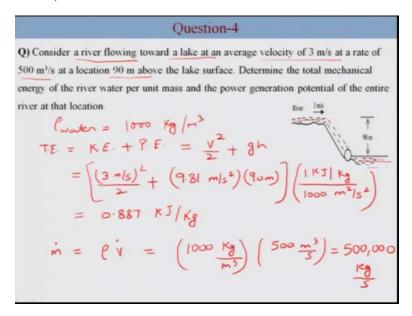
Let us move to the next problem, so next problem is about a river which is flowing toward a lake at an average velocity of 3 meter per second, at a rate of 500 meter cube, at a location of 90 meter above the lake surface. So, this is a lake, so this is a lake, the river is flowing at a velocity of 3 meter per second and the volume flow rate is 500 meter cube per second and the height of the river above the lake is 90 meter.
