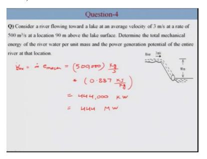
Now the work the maximum work which can be produced or generated by this water flowing in the river, so this is mass multiplied by the mechanical energy of the river. So, mass flow rate is this as calculated multiplied by the mechanical energy per unit mass of water. So, this is kilowatt or we can write it as 444 megawatts. So, this is the potential of the river, if it is recovered completely.
