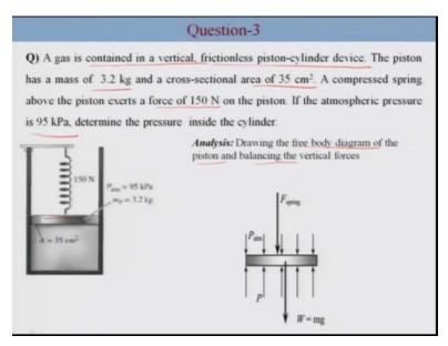
Moving to the next question, in this question the gas is containing a vertical friction less piston cylinder device. The mass of this piston is 3.2 kg and a cross sectional area is 35 centimeter square, a compressed spring above the piston. So, this is the spring which is compressed and exerts a force of 150 Newton of all the piston.
