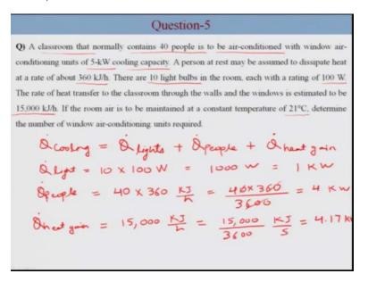
Moving to the next question which is completely based on energy balanced classroom that normally contains 40 people is to be air conditioned with window air conditioning units of 5 kilovolt cooling capacity. So, one air condition has a cooling capacity of 5 kilowatts, a person at rest may be assumed to dissipate heat at a rate of about 360 kilo joule per hour.
