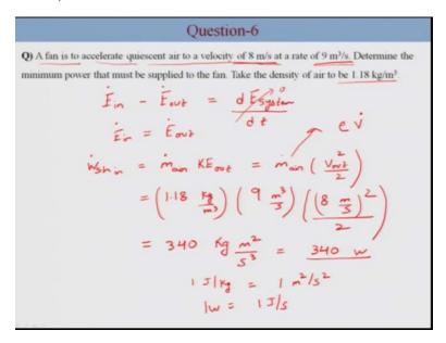
Next question deals with a fan, where it has to accelerate quiescent air to a velocity of 8 meter per second at a rate of 9 meter cube per second. So, we have to determine the minimum power that must be supply to the fan and the density of air is given as 1.18 kg per meter cube.
