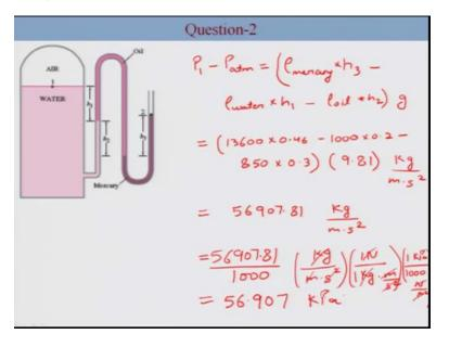
Now we have to tell what is the gage pressure? So gage pressure will be P 1minus P atmosphere. So, this expression simplifies to Rho mercury into h 3 minus density of water into h 1 minus density of oil into h 2 and completely multiplied by g and g is taken commons of. Putting all the values which are given in the question, density of mercury is 13600, h 3 is 0.46 and density of water is 1000 kg per meter cube, h 1 is 0.2 and density of oil is given 850 and h 2 is 0.3 and
