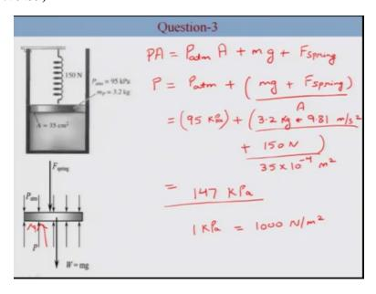
So forced balanced for this is P which is this is an upward pressure. So, P multiplied by area is the force which is acting upward. This is equal to all the forces which are acting downward. So, force due to atmospheric pressure is acting downward, so this is P atmosphere, pressure atmospheric pressure multiplied by area plus, because of the weight so weight is mass multiplied by acceleration due to gravity plus force because of the compressed spring.
