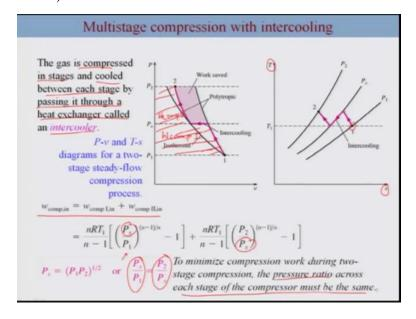
So this is the reason that typically the gas can be compressed in stages or rather is compressed and cooled between each stages by passing it through a heat exchanger which we call it intercooler and the reason is that is you reduce the temperature in order to reduce the work required for compressing the gas.
