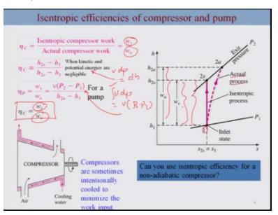
Similarly you can also find out the isentropic efficiency for compressor and pump, for the case of a compressor or pump the initial pressure is going to be low and along the process isentropic process for the idealised where there is no irreversibility ok, where is a constant entropy. So we are assuming that the actual and the idealised compressor the exit pressure is same so this is your total work for the case of idealised or isentropic process.
