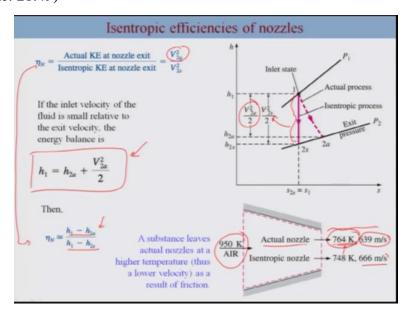
We can also extend this analysis for nozzle which are again adiabatic device and for the case nozzle which is of course an adiabatic device this are used to increase the accelerate the fluid that is increase the velocity.
