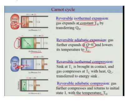
So let us consider our complete cycle, okay, for the Carnot case. So here we start with the system at one and it takes energy source at temperature Th. Remember that this Th is same as the system that means a very small difference, okay. There is no finite difference here. So heat supplied is Qh, and then it expands, this will call Reversible isothermal expansion at a constant Th by transferring Qh.
