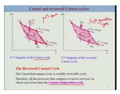
So this is PV diagram. If we go back to polytrophic process, then gava or PVn constant. So recall that slope N, if you take log P by log V, you can write in terms of slope. Typically you will see that for isothermal slope is lower than adiabatic. So this starts from isothermal expansion, then we have adiabatic expansion, then the system is compressed at isothermal condition followed by adiabatic compression, bringing back to the original condition.
