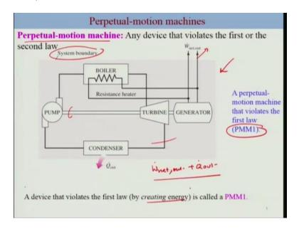
So let me consider device, what is described here. This particular device has a boiler, turbine, condenser, and pump operates on the cycle. It is supposed that the energy needed or required to heat water in this case for example can be formed internally rather than form the outside. Such as let us say, Furness.
