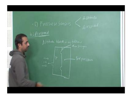
You have a chamber which is divided into two volumes by a small diaphrgram here you have a standard pressure some known pressure you are here and this vent is opened for air so the pressure difference P, pressure difference between this two volumes will be will cause deflection in this diaphrgram which will be again given to you in terms of voltages which can be calibrated and you get what will be your present altitude based on the pressure which you have got.
