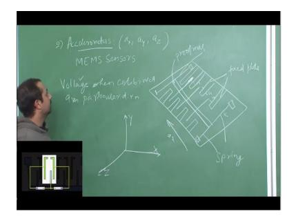
The second sensor which we talk about Accelerometer remembers when we showed to that flight required data recorded. You saw there were three times named as ax, ay, az these represent acceleration in X, Y and Z direction. Now Accelerometer the walking principle is this for MEMS sensors which use the schematic of them it will be these are your is you proof mass.
