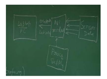
This is a basic block diagram for calibration of control surface. We have discussed about your full system what will be required for your calibration of control surface. Now what is a process for determining what calibration of your control surface? Now the procedure involves you have to first mount your inclinometer on the control surface for which we want to measure on calibrate. Once this inclinometer is mounted on that device, you have to secondly determine reference point.
