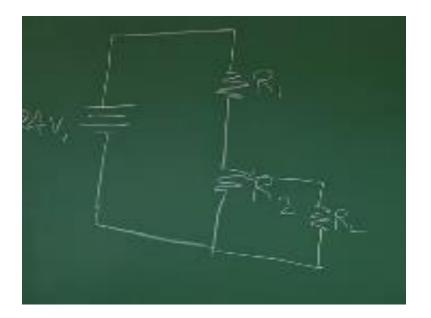
You have to determine what will be the voltage across this load resistance, which will be equal to if we further simplify this circuit.
