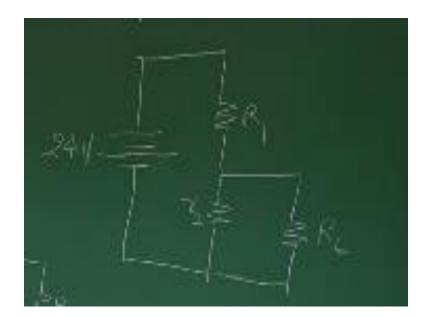
So the voltage across this load resistance will be the voltage across this RL which can be determiner using formula. The equivalent resistance between this two will be R equivalent = R2RL/R2+RL, now this will be modified as R1/R equivalent. So voltage across this resistance will be V equivalent = I\*R equivalent, where I will be V equivalent=I\*R equivalent, I=Vdc/R equivalent + R1.
