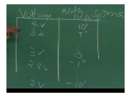
So you will get a chart with voltages and deflection of control surface. Now since we are assuming that this is a linear variation that deflection of control surface with voltage is of linear variation, so will plot a voltage vs deflection will give you positive negative. We will give you a line of sort y=mx+c.
