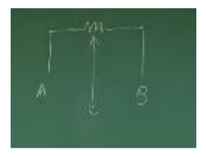
A three terminal device and it has a rotatory contact, which act as potential divided between these two terminals. These two terminals you can vary a resistance according that contacts which on your potential will vary according to that sliding mechanism. A simple circuit of potentiometer can be represented by(Refer Slide Time: 06:29)
