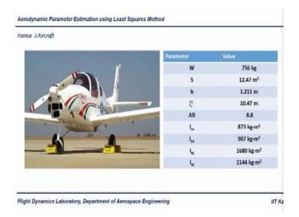
So this is air craft Hansa 3 air craft we have use to gather the data and if you see that it is a twin seated air craft research air craft so we use this for our research work. And then where it is 760kg as 12.74 meter square in span is 1.221 meter cord length is 10.47 meter as the procedure 8.8. And inertia parameters are like I X is 73kg meter square IYY is your 907 kg meter square IZZ is 1680 meter square IXZ is 1144 kg meter square.
