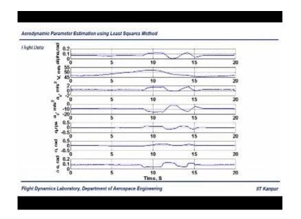
This is your geometrical parameters of this hansa 3 aircraft yes. So these are the longitudinal data we have gathered during the flying condition you see here elevated has been deflected so this is a standard signal which we say 3211 yes. So if can see the elevator which is right at the bottom here and we tried to make it like a 3211. 3211 says like it should be 3t time's upper down 2 t times if it is down then it should go up then three t times down and up.
