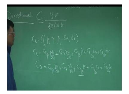
What is the directional case we long which there are less about y axis right and lateral is rolling about x axis and directional is about z axis do what is the convention for direction case right wing going back is possible so the young moment co efficient will be positive your right wing is going back okay so and Cn is the join moment co efficient and you all know how they are defined zy moment non dimensional light weight  $\frac{1}{2} \rho v^2 s x b$ , b is the span it is a usual definition.
