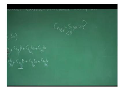
As you recall earlier lecture by plot Cn verses  $\beta$  is equal to something like this, both should be positive, this is  $\delta \phi / \delta \beta$ , for directional case, for longitudinal case, it might be Cn versus  $\alpha$  and both should be negative, right. We say Vcn, V $\alpha$  will be like this, we have understood what we earlier we call it, than we understood earlier that Cn $\beta$  should be greater than 0. Now we can say Cn data, okay, what should be the final Cn data?
