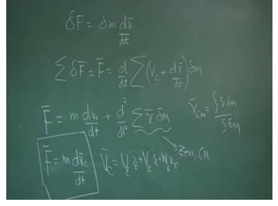
Now what do I do? I start with delta F equal to Delta MDV by DT. So summation of Delta F let me write so that I can explain it, will be D by DT of summation of VC + DR by DT. Right? I have done summation means resultant force vectoral summation and V is VC + DR by DT. So, D by DT of V is V C + DR by DT into Delta. Summation is done.
