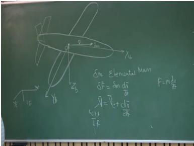
So this is YB, this is XB, body axis YB and ZB. And this is the location of Delta M denoted by R bar measured from centre of mass. What we are doing? We are trying to develop equation of motion or we are trying to apply F equal to MA using inertial frame of reference. That means, whatever measurement will be made in terms of acceleration or velocity will be with respect to inertial frame.
