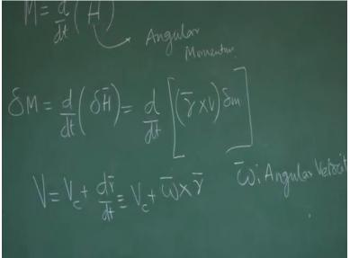
Now let us do a little bit of algebra. So H, momentum, I can write as summation of R Cross V DM which again I can write H is equal to summation of R Cross, for V, I will write VC + omega cross R. Then DM. Nothing great I have done. V I have replaced V by VC + omega cross R.
