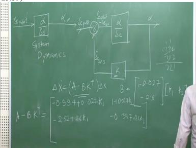
As derived earlier, for stability augmentation, the new matrix which is given as, it is X double dot equals to A - BK transpose or K as already told into Delta of X. So in this question, your B matrix is given by - 0.027 and - 2.6. Your value of K transpose or is given and K2.
