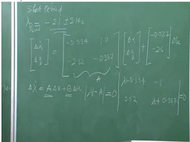
Suppose for an aircraft, the short period mode is very poor. I have to design a feedback system so that my desired root is -2.1 + -2.14I. These are the desired roots which is required by my system. Your system is given by Delta alpha dot by Delta Q dot. This is for short period. Equals to -0.334, 1.0, -2.52, -0.387 into Delta alpha into Delta Q + -0.027, -2.6 Delta of Delta E.
