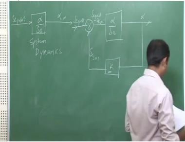
So your change of angle with respect to elevator deflection is given by transfer function alpha upon Delta E. This represents my system dynamics. Your input is Delta E which is given by pilot and your output is angle of attack. Now this is an open loop system which gives your directly angle of attack when an elevator input is given to this system.
