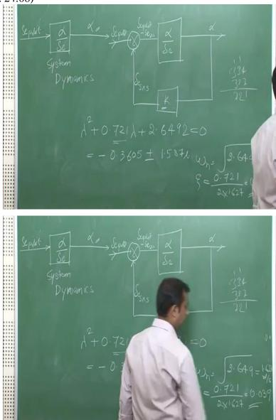
We will get characteristic equation as Lambda Square + 0.721 Lambda, + 2.6492 equal to 0. The roots of this characteristic equation equals to - 0.3605 + - 1.587 I. From this characteristic route, you can find the value of Omega N which is root over 2.649 which will give me 1.6 to 7 rad per second. And Zeta will be 0.7 to 1 divided by 2 into 1.627 equals to 0.039.
