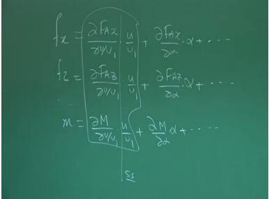
Good morning friends. If you recall, we were trying to find out the expression for partial derivatives which were required to model the perturbed aerodynamic forces and moments and if you recall, this was expanded as FAX by DU by U1 + DFAX + D alpha into alpha. Like this. Similarly, this was DFAZ by DU by U1 into U by U1 + DFAZ by D alpha into alpha and then Q terms, alpha dot terms.
