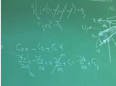
CX is equal to -CD + CL into alpha. So DCX by D alpha will be -DCD by D alpha into alpha into DCL by the alpha + CL. This is clear? Now tell me, what do we want to find out? We want
