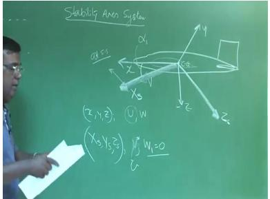
And also, very importantly, we should not forget, we are using stability axis system because the perturbed equations of motion were simplified using stability axis system. So it is important, we again try to understand what is this stability axis system? Let us say this is the airplane and this is body axis, X, Y, and Z. This is the centre of gravity and this is the wing. This X, Y, Z is the body fixed axis system.
