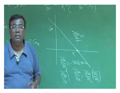
Because of static stability, when you plot it, CM vs alpha, we said there is a requirement of these airplane to be statically stable about the trim. Then the slope should be negative. So DCM by D alpha should be less than 0. So this is the condition for static stability. So typically, these values will be negative. And you know that also, you cannot go on making this more and more negative because more stable means difficult to control.
