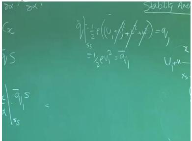
Q bar was half Rho U1 + U whole Square + V Square + W Square, all the perturbed quantities are included here. But when I write Q1, I am evaluating this at steady-state which becomes Q1 and steady-state, this is 0, this is 0, this is 0. So it is only half Rho U1 square and which is Q1 bar. 1 is for steady-state condition. So we have written this. As simple as that.
