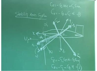
So we have no objection that this is alpha 1, this angle and we have, there is some disturbance that has happened. Because of that, total velocity has changed from the steady-state velocity. Let the component here is, earlier it was U1 at steady-state and + U is resolved along XS axis. This is a very small disturbance which is perturbed alpha. Okay? Clear? What is the message?
