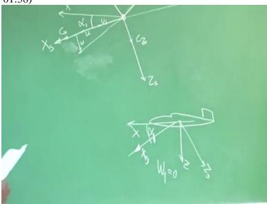
To revise your understanding, we know that this is an airplane which was having X axis like this, Z axis like this and it was having steady-state angle of attack let us say alpha1. It is cruising at alpha 2 degree. So I say alpha1. When I am defining stability axis system, I am saying I am aligning this X axis along the total velocity in the vertical plane and I am calling it XS. So naturally, your Z will become ZS. So you could see that now I am not working in X and Z axis.
