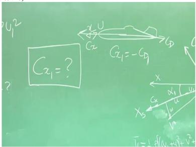
What is CX1? Let us see like this. Suppose this was X and the velocity was in this direction. Then CD would have been like this. CX is defined like this, in this direction. If the flight was like this, the condition was like this, what would have been the CX1? CX1 would have been nothing but - CD or CD1. Now let us see, in the generic sense of understanding, how do I find out what is CX1 in terms of CL and CD? Please understand we are trying to find out everything
