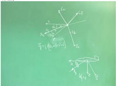
So if I draw the diagram for more clarity, you could say that this is alpha1, this is X what I was showing here, this is the perturbed U, this is the steady-state value U1. With that is the XS direction. And now because of disturbance, total velocity direction will change which is given here, let us say V Star. Total dynamic pressure will be now, if you see, ideally speaking, total dynamic pressure will be half Rho U1 + U square + V square + W square.
