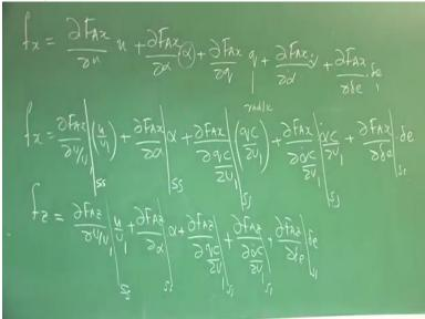
Let us say, we take FX. FX is what? It is DFAX by DU into U + DFAX by D alpha into alpha + DFAX by DQ into Q + DFAX by D alpha dot into alpha dot + DFAX by D Delta E into Delta E. Let us take first this case. Let us also see, what are the dimensions of alpha? Alpha is angle. It is dimensionless, radian. Q is radians per second, alpha dot is radians per second, Delta E is dimensionless, U is m/s.
