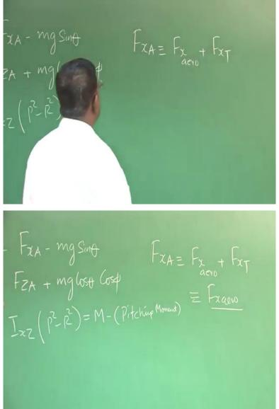
What is FXA? If you see, FXA is actually equal to FX aerodynamic + FX because of thrust. Similarly FZA is FZ aerodynamic + FZ because of thrust and M is nothing but pitching moment. This is nothing but pitching moment. To make our life simple, we will make an assumption that whatever treatment I do for FXA, it assumes that as if FXT is not there. Or whatever treatment I do for FX aero, similar treatment could be made for FXT.
