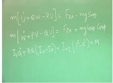
And if I recall, we had equations of motion of this form. MU dot + QW - RV equal to FXA - MG sin theta. This is one of the equations and along Z direction, the equation was MW dot + PV - QU equal to FZA + MG cos theta cos Phi. And the pitching equation was IYQ dot + RQ IX - IZ + IXZ P square - R square equal to M. Now we need to understand the right-hand side.
