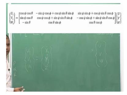
So using these 3 rotations, we can convert our frame from initial frame to the body frame or body frame to inertial frame. We can combine all these rotations in one equation. We will get in inertial frame, all 3 velocity components and this can be given by the multiplication of 3 matrices. This U, V, W is in body frame and by multiplying this matrix, we are able to get U1, V1 and W1. This is now in inertial frame and this is our desire because we want to find the trajectory.
