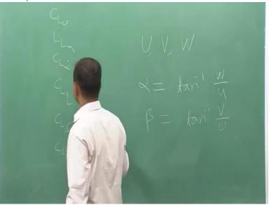
If the velocity component of the aircraft in the body frame U, V and W, the angle of attack, alpha will be Tan inverse W by U and beta will be Tan inverse V by U. So now if you have the alpha and beta and all the forces, lift force, drag force and Y force, then using these 2 angles, you can find F aerodynamic X and F aerodynamic Y and F aerodynamic Z acting in the body axises in the aircraft.
