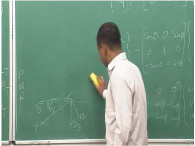
In this third rotation, you will get the matrix 1 0 0, 0 cos Phi - Sin Phi, 0 Sin Phi and cos Phi. In third rotation, we have front view of the aircraft. If this is my front view, suppose this is our Y3 and this is Z3, for this rotation, for the positive Phi, the right wing down is the positive Phi. So, right wing down means if this is my front view, it will be like, it will become like this and this is my final Y and this is Z. And this angle is Phi.
