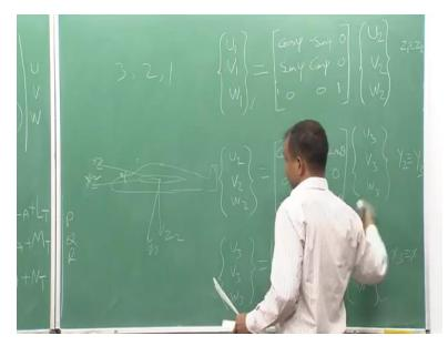
We can write in matrix form, this rotation. Suppose our velocity component in inertial frame, U1, V1 and W1. And after the Psi rotation, it becomes U2, V2 and W2. This U2, V2 and V2 in intermediate frame and this we got after the rotation, Psi. We can write this matrix, cos Psi - sin Psi 0. Sin Psi, cos Psi 0. 0 0 1. And second rotation, we rotate about the new Y axis and using that rotation, you can get U2, V2 and W2, U3, V3 and W3.
