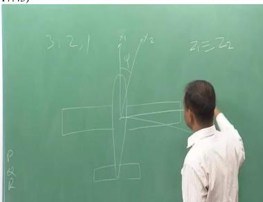
But in Euler, we used the sequence of rotation, 3, 2, 1. First, we rotate our frame about Z axis. Then, the new Y axis which we got after the rotation in the Z axis. And lastly, we rotate our frame about the new X axis which we got after the second rotation. Let us see it. Let us say I have top view of my aircraft.
