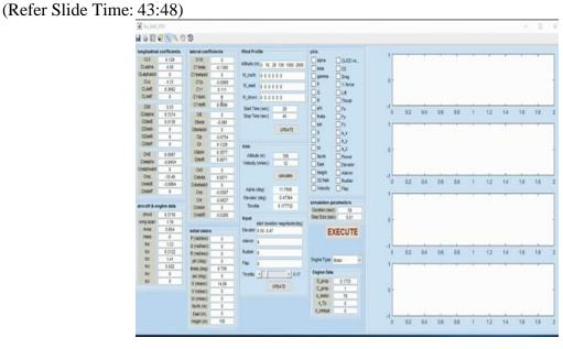
We have developed a crystal user interface for 6 degrees of freedom simulation. In this, here you can feed all the aerodynamic coefficients associated with the longitudinal motion, the lift coefficient, drag coefficients and the pitching moment coefficients. In this window, all the aerodynamic coefficients associated with the lateral and directional motion of the craft, coefficient for the Y force, all the rolling coefficients and plain coefficients.
