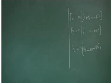
So for our ease of communication, I write FX is equal to M U dot + QW - RV. FY equal to MV dot + UR - WT and FZ equal to MW dot - UQ + VP. We have not asked this question, what are these Fx, XFY, FZ composed of? We will come to that question. We have most focused on the right-hand side, what are the kinematics for this? Now, we also have to handle the other equation which is the moment equation. Let us do that.
