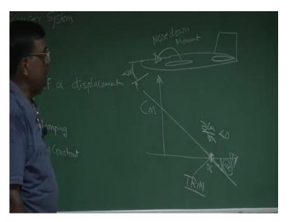
So if this is is more than 5 degree, it should generate a nose down moment. We all know that and that is how we draw CM vs alpha and the slope, DCM by D alpha negative. If at equilibrium, DCM by D alpha is negative, we say the body is statistically stable. No doubt about it. We can again crosscheck here. If the airplane is flying at this trim, why this is trim? Why do you define this as trim? Trim means, the CM is 0.
