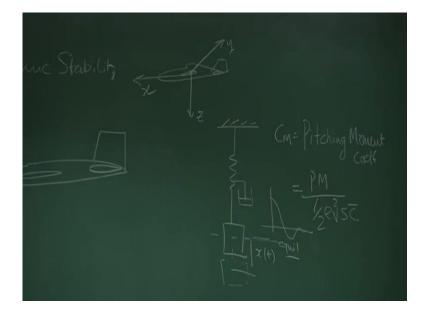
And to be more explicit, if I draw the airplane like this, if this is the x-axis and if this is the y axis, and this is the z-axis which is the body fixed axis? Pitching moment is motion about Y axis. Nose up is positive, nose down is negative.
