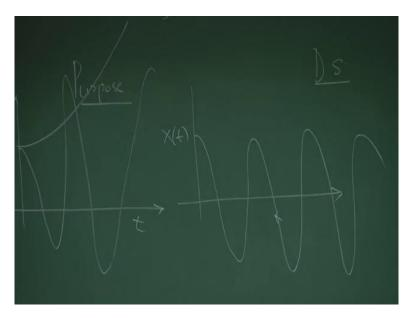
There could be a case where see, this is the disturbed quantity. This is time and this man goes on oscillating like this. You see that amplitude is not increasing but it is going on holiday. So it is actually speaking, dynamically neutrally stable. So this sort of cases, we will be discussing and this sort of understanding of the definition is required and what is the response here?
