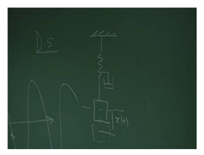
If we see a similar example for a mass spring damper system, once I disturb it, this distance is XT. This is a perturbed point, small perturbed. Right? The perturbation should be such that three should not be any gross stage in the whole system behaviour. In the sense, I should not stretch it so much that the spring constant will change, the length of the spring will change, the material cross-section will change. All these things are not allowed. Okay? That is a small disturbance.
