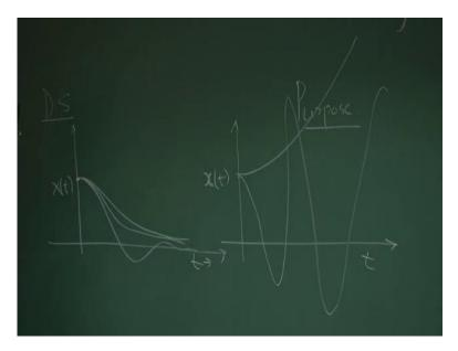
Even system is dynamically unstable. Then if I have given a disturbance, it may go like this, it may go like this, it may go like this. All are simply representing that system is dynamically unstable because in finite time, the disturbed element or disturbed motion variable is not coming back to the equilibrium.
