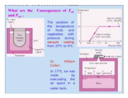
The consequence of saturation pressure and temperature right let me just tell you that this temperature as I told that saturated temperature will be dependent and pressure and vice versa right so if you look at like suppose can I use this thing for producing eyes right or cooling it and how we can do if you look at like what I will do I can go on reducing the pressure right when I
