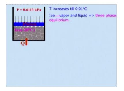
That means all the three phases will be at the same point you know it will be simultaneously being present so this is a very important point I had emphasized in the last lectures that this triple point was being used as a reference point for the temperature measurements high temperature scale to make it that because it is invariably there is small change in that temperature then you know you would not get three phase you know immediately.
