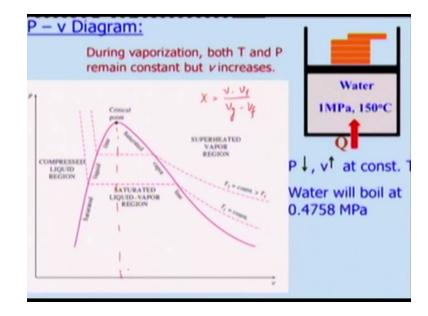
The piston and cylinder arrangement and where we will take a water and at one mega Pascal's and 150<sup>°</sup> Celsius and we will take our this is our system and it is if you look at it is already loaded with tiny weights and if I remove this small weight what will happen to this water which is had 150 degree Celsius you know at one mega Pascal. What will happen? If I remove this way the pressure will be decreasing.
