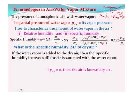
If water vapor is added to the air then specific humidity of course will increase right till whittle it attains the saturated condition right and once it is saturated you cannot really change that unless you change the temperature right because in atmosphere you cannot really change the pressure that much but temperature can go up so therefore we need to know that what is the relative humidity.
