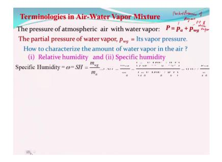
And can write down that as by using the ideal gas law that is p wz into v volume is the same into molecular weight of water into / re 1 t and similarly for air I can write on the using ideal gas law that is PA v molecular weight of air/ r UT if you look at like this the same temperature because the air will be at the weight air will be at same temperature right so therefore this will be cancelled it out right.
