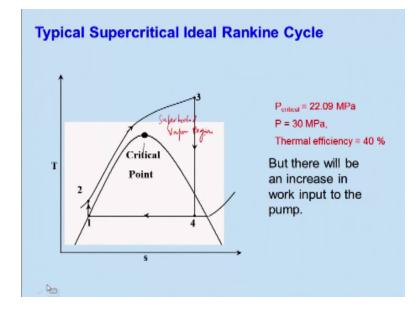
So there is another way of going by that that if you go on this pressure right if I go on increasing the boiling pressure I can reach a point critical point right, if I increase that critical point then like it will be a go directly the liquid will be converted directly into vapor this is your superheated vapor region right. So that what happened I can compress this and then go directly into the point 3?
