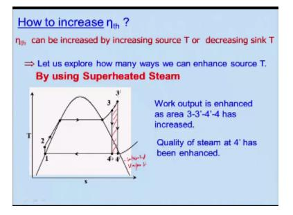
And so then question arises how to increase the thermal efficiency of the Rankine cycle what are the ways and means if you recall that when we are discussing about the Carnot cycle I had told that you can increase the thermal efficiency by increasing the source temperature right or by decreasing the sink temperature. So that is the way where we can increase the thermal efficiency for the Carnot cycle and a similar way also we can do for the Rankine cycle.
