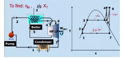
So let us consider an example like in a thermal power plant operating in the reheat cycle steam at 50 bar and 500°C this pressure is given 500 I mean here itself one can say that it is superheated steam right, it is not saturated enters into a high-pressure turbine and leaves it at 10 bar right, and the steam is reheated back to the 500°C that is a restriction for this power plant before being fed into low pressure turbine condenser is maintained at 0.05 bar, right.
