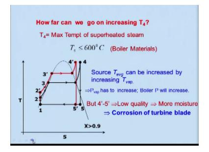
So therefore the quality has also improved. So question arises how far we can go on increasing the temperature 4, the maximum temperature, temperature 4 state 4 means the maximum temperature right, there is a limitation of that is metallurgical limitation that is the, like being done, because it is generally restricted to the 600°C that means it will be less than equal to 600°C as of now.
