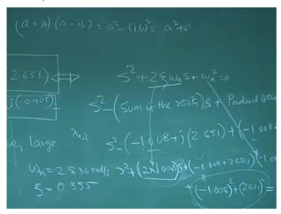
If I take this since I have seen this is at typical second order response so I write this as characteristic equation as s square + 2 get a omega n s + omega n square = 0 you know this is typically second order characteristic equation in terms of omega n and zeta and so I construct this equation from this root this form. So I write s square - sum of the roots into s + product of the root equal to 0.
