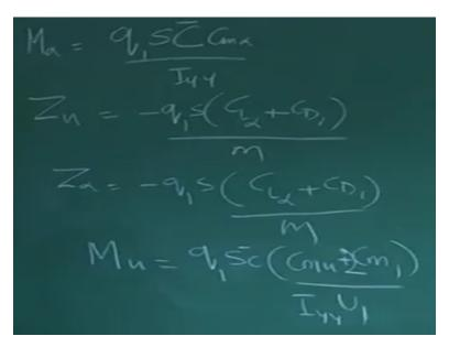
So this is the condition. Question is what does this tell us? Let's go back what was m alpha. M alpha was defined as q 1 s c bar c m alpha by I y y and then second term is z u, what is this z u expression is - q 1 is C L alpha + c d 1 by m and what is your z alpha z alpha is - q 1 s C L alpha + c d 1 by m and what is m u. mu is said to be q 1 s c bar cmu + c m 1 into c m 1 I y y u 1, right.
