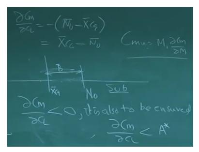
So what is dcm by d c l we have see dcm by dcl is nothing but - starting margin that is - x or - neutral point - x c g bar or we can write as x c g bar - n not bar. N not is the neutral point. For subsonic case what is just simply telling is that if this is the n not ok. Aircraft will be subsonic right from there what I am saying getting is dcm by dcl should be 0.
