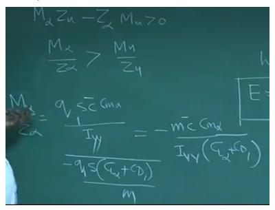
So e greater than 0 means we will see that m alpha z u - z alpha m u greater than 0 that means m alpha by z alpha greater than m u by z u. We are seeing that we are trying to understand what additional information relating to stability we are getting through this coefficient. We know for dynamic stability all this A, B, C, D, E should be greater than 0 so you are studying a case for E greater than 0. e greater than 0 means this expression greater than 0.
