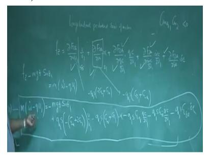
If I do that you know the equation of motion is fz - mg theta sin theta 1 equal to m w dot- q v 1 right. We have to substitute fz using this expression and using the value of expression for all this term. For example for dfz by du1 will put minus q1s and 2cl 1 + CLU right. Dfz by d alpha will put -q1 s + cl alpha like that. For dfz by dq was cl also like qc by 2v1.
