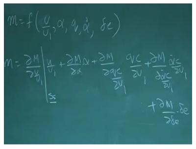
Now you are expert m in write function of alpha and or u by u1 alpha u alpha dot delta e ok. What is next so mu writes us dm by du by u1 into u by u1 + dm by d alpha into alpha + dm by dqc by 2u1 into qc by 2u1 then dm by d alpha dot c by 2u1 into alpha dot c by 2u1plus dm by d delta e into delta e ok. These are the equation for this expression or oscillating pitching moment
