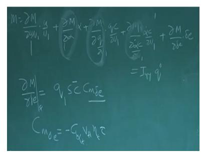
We have written m is equal to dm by du by u1 into u by u1 + dm by d alpha into alpha + dm by d qc by 2u1 into qc by 2u1 + dm by d alpha dot c by 2u1 into alpha dot c by 2u1 + dm by d delta e into delta e ok. We have developed expressions for all this derivatives for example if I take dm by d delta e which is nothing but q1 s c bar cm delta e and we know the expression for cm delta e we might have seen in initial lecture.
