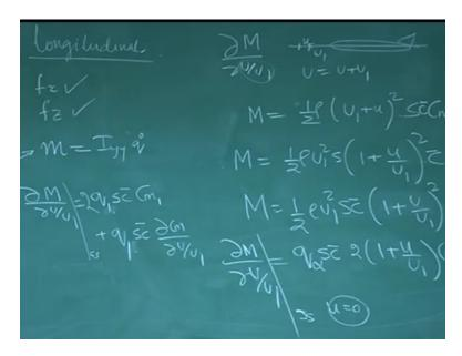
For longitudinal case well we have already seen the equation along the x axis has been completed, along z axis has been completed along x is this and along z is plunging. Now what is remaining is pitching. Because you know we are talking about longitudinal perturbation. That is perturbation is man aircraft will do like this and the passage will go up and down and the velocity along in also is reduced.
