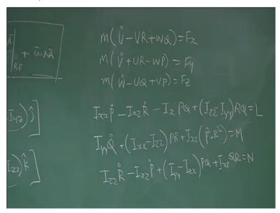
To be seen m u dot minuses u r + w q is equal to fx and you know m v dot + u r minuses w p is equal to fy then m w dot minuses u q + v p is equal to f z if you do this operation and do the I x x p dot minuses I x z r dot so without the fxfy and f z right here from once set of equation and need to do this cooperation we will got equation like this I x z r dot minuses x p q + I z z minuses I y y into r q the component of movement.
