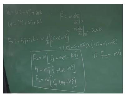
What we wanted was F equal to m dvc by dt in initial frame and now we know that. That is equivalences in m dvc by dt in body frame or rotating frame and comma omega cross vc for this equivalent to working in body frame right. It is the initial frame we are not expecting in this. What is VC please understand in body frame then + vj in the body frame wk in body frame we working in body frame please understand this right.
