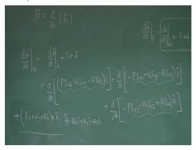
So we know need to calculate m as d/dt(h) angular movement of vector .so I lose this dh / dt in initial frame will be equal to I find dh / dt . and dh / dt in the body frame + omega cross h and you know h vector as to be expressed in body frame you know the component of h a h so I specify hd / dt or of it me write p I x minuses q I x y minuses r y z and this is now I that is in the body frame .
