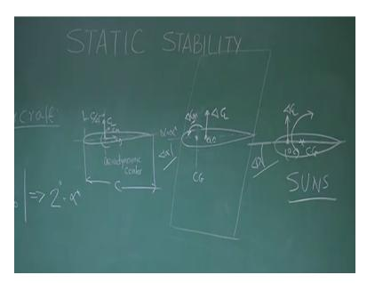
So that is how static stability is assured you can immediately see that, if this is the aerodynamic center and if CG is behind aerodynamic center or I say aerodynamic center is ahead of center of gravity.
