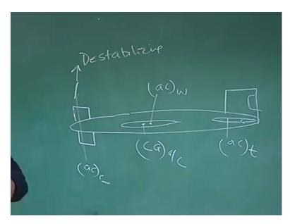
Suppose this is an airplane, let's say this is CG of the aircraft, and let us see AC of wing and of course this is AC of tail okay, let's say this is the configuration, again I am assuming fuselage contribution is neglected. If I see this I could easily check as, AC of the wing is behind CG of the aircraft, so this will give stabilizing contribution, a new AC of the ac of tail is behind the CG of the aircraft, this also give a stabilizing contribution.
