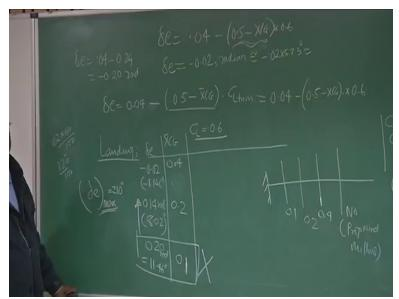
And, if I now simplify what do I get? So I get Delta E = 0.04 then, + N 0 is 0 point 5 - XCG bar divided by - 1, so CM Delta is -1, so I put it here a minus sign into CL trim right. Now see this case think of landing, so when I put N 0 = point 5 because, I am studying a case landing that means I am clear that this is propeller wind milling case okay. Let's see this point 5, now let us do a tabulation, I want to see what is the effect of moving CG forward for Delta E required.
