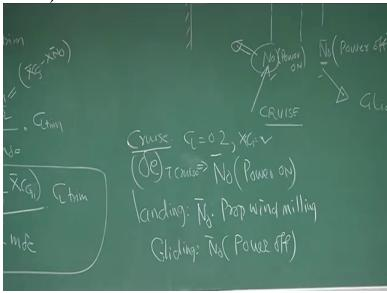
Now let us say suppose it is coming for landing that is what is the case of landing? Propeller wind milling right N 0 should I use I should use N 0 propeller wind milling so it will be N 0 should be corresponding to propeller wind milling okay. Suppose we are coming for gliding, right we want to glide switch off the engine, and we are not allowing propeller wind milling are you simplified case suppose I am doing a gliding flight with the glider.
