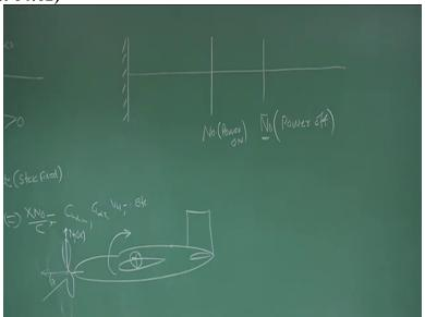
What is important here is that we have not incorporated any effect of engine right. So, now what we find is if I draw a line like this and if this is my reference we say N 0 some time I write XN0 or N 0 they are same when I put N 0 bar means N 0 non-dimensionalised with chord with mean aerodynamic chord right. Once we have calculated N 0 we some time I write it as XN0 or N0 bar bar means by now you that it is non-dimensionalized with mean aerodynamic chord.
