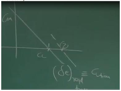
Suppose this is my CM versus CL I am flying here this 1 and to fly at 2 I want to know, how much elevator I should deflectrun so that, I can again trim at CL 2. So relationship between Delta E required some term we say Delta E trim and CL trim is what is a control problem for this flight mechanics what we are discussing, how do I formulate it?
