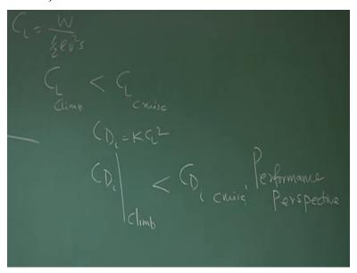
If it is climbing so this CL climb is less than CL cruise what is the implication of this? In a performance we have seen it means the induce drag CDI which is KCL square that means induce drag CDI for a climb is less than CDI for a cruise, that is a drag coefficient okay. CDI for a climb is less than CDI for a cruise this is from my performance prospective no issue right.
