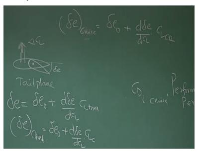
So if I want to know what is the Delta E required for climb I should replace so I write Delta E during climb will be = Delta E0 + D + Delta E by DCL into CL climb CLC.
