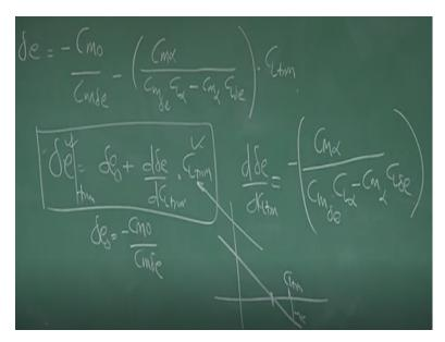
And that will be Delta E = - CM0 by CM Delta E - CM Alpha by CM Delta E into CL Alpha - CM Alpha into CL Delta E into CL trim let me check, - CM0 by CM Delta E - CM Alpha by CM so I can write this Delta E = Delta E0 + D Delta E by DCL trim into CL trim where, D Delta E by DCL trim is nothing, but - CM Alpha by CM Delta E CL Alpha - CM Alpha CL Delta E right. What I have done, this whole what is Delta E0 from this expression very simple CM0 by CM Delta E.
