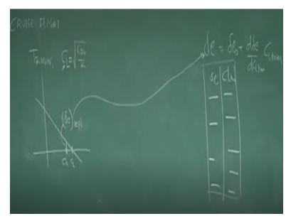
This is one understanding. Second 1 once, I write Delta E = Delta E 0 + D Delta E by DCL trim into CL trim. I am knowing that for CL trim for this CL trim, this Delta E required for this CL trim this Delta E required like this you know, so pilot will develop a field from the Delta E, how much Delta he required to give for the CL trim or he thinks in terms of he gets the feel in terms of speed, so your giving Delta E and speed that's sort of mapping you're doing for a pilot okay.
