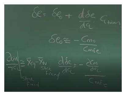
So you know Delta E = Delta E 0 + D Delta E by DCL into CL trim and Delta E 0 was approximately shown to the - CM 0 by CM Delta E and D Delta E by DCL was - DCM by DCL by CM Delta E. I am putting a approximation because we have neglected few terms okay. So what is the message for an airplane Delta E 0 is known because airplane will have a fixed CM0 and CM Delta E, if it is low speed airplane.
