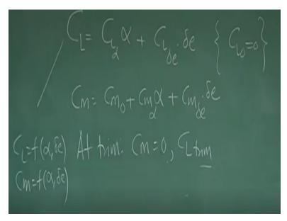
E, for simplicity I have put  $CL \ 0 = 0$  you can introduce  $CL \ 0$  here and do the derivation, and most likely I will be give in that assignment. Then CM will be  $CM \ + CM$  Alpha into Alpha + CM Delta E into Delta E we are clear? Because here we have seen CL is function of Alpha and Delta E, we are not talking about any dynamic condition so, since CM has come because of CL CM also will be function of Alpha and Delta E, so CL have expanded in the linear way.
