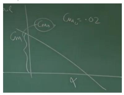
Our aim is to ensure that CM versus Alpha or CL graph, if its Alpha this is CM0 I need to have this CM0 desired, for example if I need CM0 = point 0 2 then, CM 0 because of wing because of fuselage because of tail so totally give me the value 0.02 okay that is important. So know what we are seeing what is CMAC wing? Because we are trying to find out what is the contribution of wing towards CM0 of the whole aircraft right?
