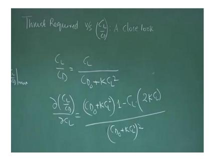
So, this is thrust required versus C L by C D a closer look. Let us see, we are very comfortable writing this W by C L by C D and this means, thrust required minimum implies, I must fly at C L by C D maximum. Let us do little bit of algebra or some sort of a and little mathematical insight into this C L by C D max. See, you know C D is C D naught plus K C L square and we know that, this is parasite drag and K C L square is the induced drag, all these things are very clear to us.
