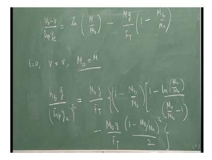
So, if I go back to the equation B, let me first write equation B here and then I will replace. Equation B was V b by I s p g e, which are this term was del V delta V, but V 0 was zero. So, this becomes equal to V b equal to l n M, just a second this will be V b by V we are starting from particular velocities of V b and then going towards V. So, this is becoming V b minus V by I s p g e.
