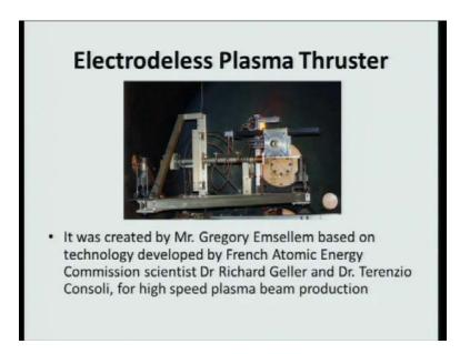
First, let us look at the electrodeless plasma thrusters. It was created by Mister Gregory Emsellem based on technology developed by French atomic energy commission scientist Doctor Richard Geller and Doctor Terenzio Consoli for high speed plasma beam production. So, the initial aim of the French atomic energy scientist, were to produce high speed plasma beam, which was then modified as a plasma thruster.
