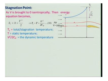
It will move away from the aero foil and keep in mind that air is going over this aero foil at a velocity inlet velocity or stream velocity of 100 meters per second. Now, if this fluid you know we will be taking, it will be going in a streamline kind of thing. If I take this fluid elasticity over here, if you look at the leading age it will come to a; what you call stand still. So fluid element has brought to 0 velocity. If I take, of course somewhere here, then fluid will go over like this.
