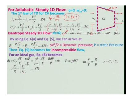
So, if I convert this equation in terms of what you call temperature what I will do I can write down in place of enthalpy I can write down Cp T 1 plus v 1 square divided by 2 is equal to Cp T 2 plus v 2 square divided by 2. How could I write this under what condition I can do this can anybody tell me we are assuming as an ideal gas right what kind of ideal gas it is. It will be calorically perfect gas because the Cp is a function of temperature, Cp is also a function of kind of fluid.
