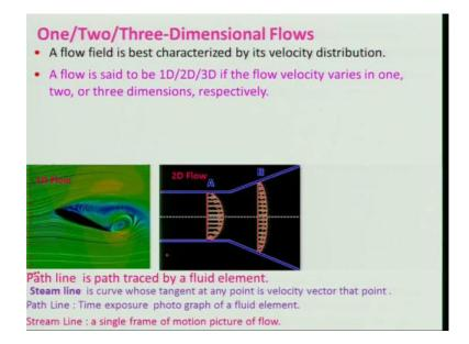
Generally, that means under steady state condition steam line or path line are same so we generally try to conduct experiment like this to what you call such that we will have a steady flow and steam line path line can be same. These are very important concept if some of you may not have a what I have seen it is you are getting confuse so it is very important to know about it.
