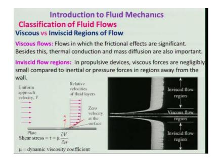
So, let us look at like when you talk about this fluid how to classify the fluid flows because we will be more interested in the fluid flow in case of this aerospace applications. How because how this fluid flow will be helpful it can be helpful in two ways one way that whenever, fluid is flowing through a duct or over a surface it will be experiencing what we call certain force will be applied, or certain force, or the thrust you
