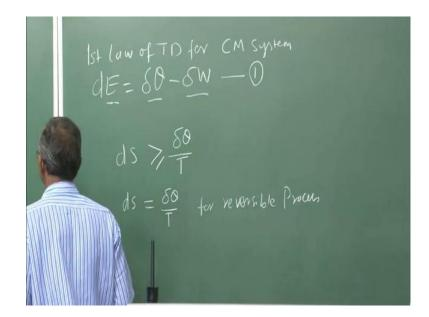
And this is basically first law of thermodynamics for a control mass system if you look at in this case this E is basically the total energy and which will be consist of both macroscopic and microscopic form of energy. Whereas, this macroscopic form of energy which we always put in terms of internal energy and macros, we form we are considering only two kinds one is potential energy other is kinetic energy, but beside this there are several other forms of energy as well.
