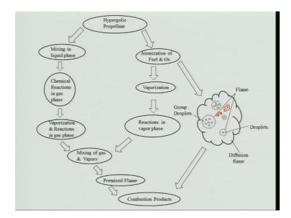
So, let us look at hypergolic propellant, the mixing in liquid phase will take place and chemical reaction in the gas phase go on is likely to occur, because is a hyper hypergolic in nature. So, vaporization reaction in the gas pressure also will be occurring simultaneously, so this all processes whatever I am describing will be occurring simultaneously, not that one will occur like that way arrow is given.
