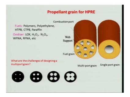
For example, fuels you can use polymers, polyethylene HTPB, CTPB, paraffin several other fuels whatever you use. And oxidizer like a liquid oxygen what you call, hydrogen peroxide, nitrogen tetra oxide, white fuming nitric acid, rate fuming nitric acid that are the several other liquid. Keep in mind that lot of interest in western countries to have their own, even in the universities of having hybrid rocket, example several universities in USA having their own systems, students had been there.
