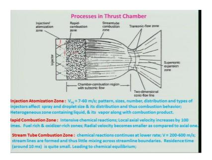
So, let us look at what is happening in the processes in the thrust chamber, if we look at we have seen the rocket engines and then, it can be like injectors head are here, and it is having you know like a two phase flow kind of thing heterogeneous, mixtures will be there. And there will be also the velocity with which it will be coming is something coming 7 to 6 meters per second, and if you look at the combustion here will be depended on the spray quality.
