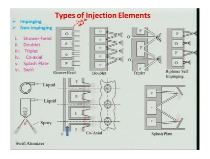
Now, I will be now talking about what are the kind of atomizer, one will be using in a kind of rocket engines, so there are it can be broadly divided in two categories. One is impinging atomizer, other is non impinging mostly the impinging atomizer being used, in case of which propellant liquid propellant definitely, but non impinging also will be using for non liquid propellant.
