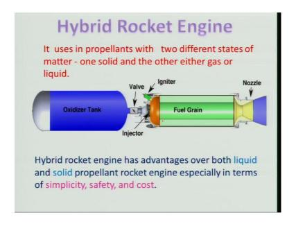
So, what you call we will be now looking at the hybrid rocket engines, and which is being used basically to have a better control, and it is quite simple and safety kind of thing. Where will be using the fuel, if we look at this are the fuel grain which is being
