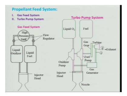
So, you can use this for finding out alpha and then, other play around this thing about the mass flow rate, the delta a P and then, look at what will be MR ratio you can use the other design tool for it. So, let us look at propellant feed system, we talk about injectors and atomizer how to go about it, but we have not looked at how to feed this, because we need to have a pressure, otherwise we cannot feed.
