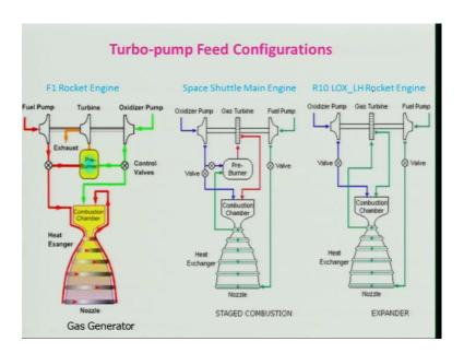
There are the three types, but there can be several other types as well, one is gas generator, if you look at it is having fuel pump and oxidizer pump, which is run by the turbine. And in this case the fuel being separated one line goes to the pre burner, and other line goes to the what you call rocket engine which will be cooling and then, it is
