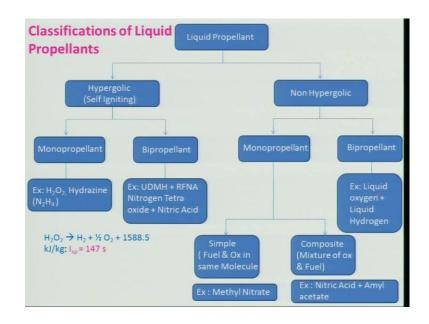
Liquid propellants basically can be classified into 2 categories, one is hypergolic propellant, hypergolic propellant means self igniting; that means, you need not to give any ignition energy for initiating the combustion. Do not you think it will be very you know hazardous to do that, because if I will have to one is fuel and oxidizer or then it will just go, then it will be start react.
