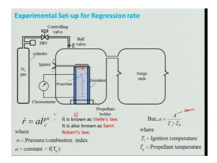
But however, experiment is being conducted, keep in mind that in experiment being conducted under a steady state, there is no flow conditions in actual situations flow will be there and several complex. Here, it is a steady state, you use a burner which is a propellant here and having insulation, it is having a propellant holder and it is in a chamber, and I can use this pressurize this chamber, with the help of nitrogen, of course controlling valve and ball valve.
