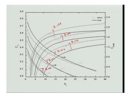
And if you look at the C c I am in like a core engines, like you will find that C c is basically decreasing right, as it is with the pie pressure ratio it sorry that C c it goes on increasing and reaches a certain values, at the higher pressure ratio compression. And the real case as I told it is a solid line is having a lower value, as compare to the ideal one which is a dace line for a particular condition. And of course, as it is decrease that this one basically t is equal to 0.8.
