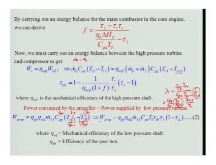
So, the carrying out the energy balance for the main combustor in the core engine, we will get the similar expression as have shown here, like this is same for both turbo fan, turbo trap, turbo you know jet engines. So, we need not to really do anything, but this is the very important part we must look at it because, the energy balance between high pressure turbine and compressor. And also will be looking at the energy balance between the low pressure turbine and propeller.
