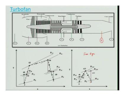
So, we let us just keep this in mind these are the turbo fan symmetric with the station number 0, 2 and of course, there is 13 for the fan, and 19 for the fan that the nozzle and the station 3 to 4 is combustion chamber of course 2 to 3 in the case of core engine is the
