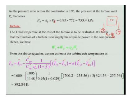
So, as the pressure ratio across the combustor chamber is 0.95, so you can get basically P t there is pi b, pi b is 0.95 into P t 4 no P t 3 this will be P t 3. Now, P t 4 will be basically pi into P t 3 because, pi b what P t 4 by P t 3 station number, if you look at combustor chamber right it is 3 and this is your 4. So, pi b will be P t 4 by P t 3, so P t 3 is equal to pi b into P t 3 right 0.95 into 772 that will be little lower than the P t 3 that is 733.4 kilo Pascal.
