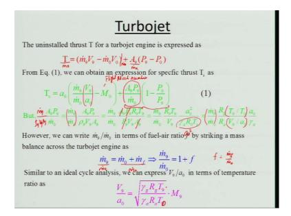
So, the uninstalled thrust for the turbo jet engine is expressed as we know that T is equals m naught 9 V 9 minus m naught V naught this is due to the momentum. You know change of the flow and this is the pressure thrust A 9, this is the area of the nozzle exit and P 9 minus P 9 and we had neglected this term pressure trust. That means, we are
