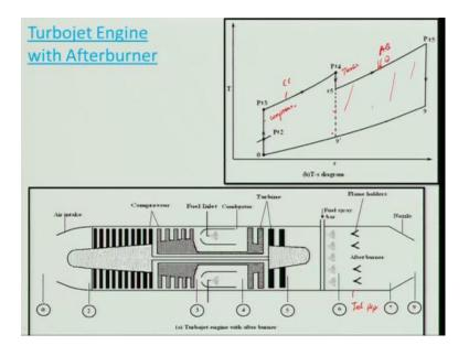
So, let us look at a simple turbojet engine with an afterburner, if you look at the fuel spray by the air, it is having fuel being sprayed and it is you know gutters are there or the flame holders various kinds of flame holders, which will help you in stabilizing flame. This is basically jet pipe right jet pipe which is there and then it will be expanded in nozzle. So, if you look at the processors what we are looking at it, of course 0 to 2 and
