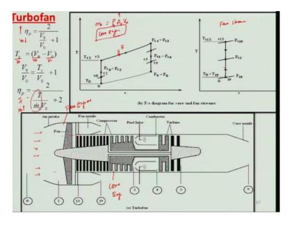
Let us look at the definition of propulsive efficiency for the particular flight Mach number or a particular flight velocity V naught, how can I enhance this propulsive efficiency given under ideal condition when I am when I am decreasing the V 9. That means if I decrease this exit velocity from nozzle, you know then only I can what you call enhance that means when V 9 will decrease the propulsive efficiency will increase.
