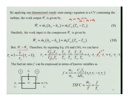
So, which will be quite simple to derive these expressions and that is very important; we need to now relate this turbine work into the compressor work, because we will have to get the relationship between the compressor and turbine. So, we will assume the one dimensional steady state energetic way, you know these things. We apply this to a energy equation control volume and the turbine work will be m dot 5 is equal to s t 5 minus s t 5, because the in the turbine.
