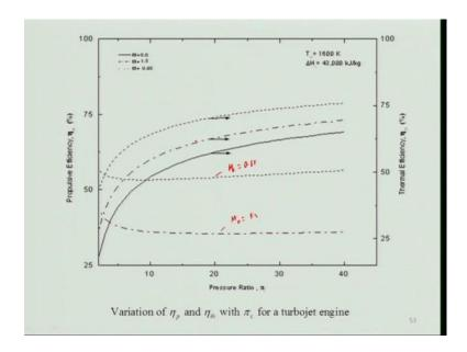
So, let us look at a propulsive efficiency and the thermal efficiency if you look at these are the curves which is you know basically the propulsive efficiency. These two curves and it is a static condition there will be no meaning of having propulsive efficiency even Mach number type number is equal to 0. So, what you call this one is basically Mach number of 0.85, it is having higher propulsive efficiency as compare to 1.5.
