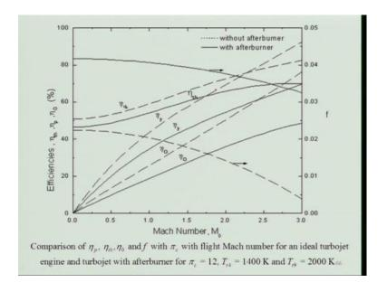
If you look at what really we are gaining in the propulsive efficiency and propulsive efficiency if you look at it is decreases because the exit Mach number exit velocity from the nozzle will be increasing. So, the heat will be decreasing and overall efficiency of course the thermal efficiency will be what you call increases. When you add this, you know when you add without any afterburner that is higher values than that of that with afterburner.
