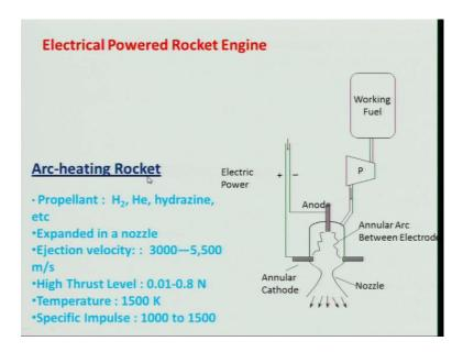
So, let us look at arc heating rocket engines, and in this case arc is being use having a in this schematic a annular cathode, and anode is being use to produce a arc, and you know that arc can be produce when the high voltage, you know will be across this cathode and anode will be there, and which will be creating a kind of a plasma as such, and because that will be broken out and a spark will be produce.
