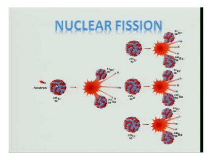
And a during the passes of fission what happens is that the uranium 235 will be observing a neutron, and when it absorbs it will be having energy level will increasing, and then it will be separated or splited into two nuclear. One is krypton and other is barium, and it will be also generating a large amount of energy beside this the gamma raise
