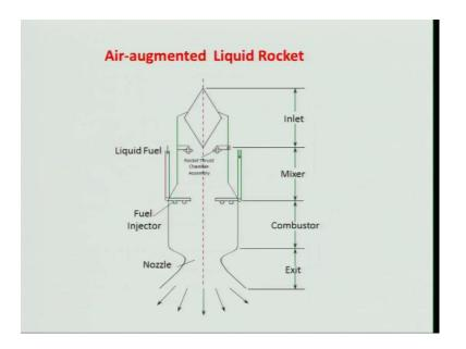
So, let us look at the augmented air augmented liquid rocket engine in this case it will be similar in nature, but; however, there is a little difference there will be a rocket trust chamber, which will their, which is not being shown in this diagram, and you will take the air all the time.
