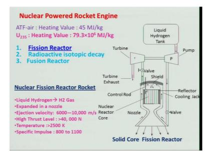
So, for rocket engineers concern. So, which will be I will be giving you only one example that is solid core fusion reactors. The schematic is being shown here, and here you can use any other propellant like kind of thing.
