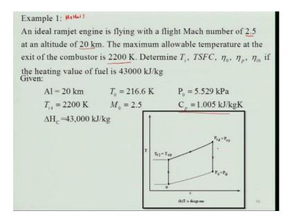
I would take the same example and used another method you can say this is the methods one and I am doing that. Now, this method, so what is that an ideal ramjet engine flying with a flight Mach number 2.5 altitude of 20 kilometer, maximum allowable temperature is 2,200 Kelvin. We will have to determine specific thrust plus fuel consumption and all other efficiencies and these are the given like altitude is given and temperature t 4 all those things i have already talked about and C p.
