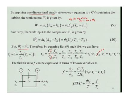
So, which will be quite simple to derive this expressions and that is very important; we need to now relate this turbine work into the compressor work, because we will have to get the relationship between the compressor and turbine. So, we will assume the one dimensional steady state energetic way, you know these things. We apply this to a energy equation control volume and the turbine work will be m dot 5 is equal to s t 5 minus s t 5,
