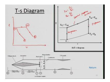
So, let us look at how what are the process that are involved as you told that zero to two is basically the compression in the t s diagram I can write down zero to two that is the compression right isentropic process isentropic compression. But if I look at in a p v diagram how it will be compression process zero to two into it will be right and then T t two from this station to what you call four it is the compression that is constant pressure combustion right.
