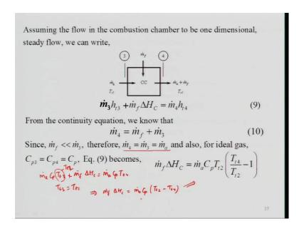
So, now we will have ti equal to look at the combustors and keep in mind that we are assuming the in the this combustion chamber the float would be one dimensional, but in real situation it can never be and we are assuming that certain amount of air is entering and and fuel being added and it is going out with certain mass flow rate of air and fuel So, we can carry you know like considering the float to be one dimensional and steady
