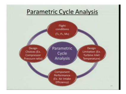
So, let us look at how we can carry out this parametric cycle analysis that means what we will be doing we will looking at parametric cycle analysis, first we will be considering ideal cycle, then we will be considering the real cycle. So, as I told you, parametric cycle analysis is very important because here the flight conditions like altitude flight velocities, when I talk about altitude, it is basically the temperature and pressure at a particular altitude which will be varying.
