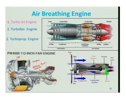
So, let us look at turbojet engine and we is really happening here, turbojet engine is having various components, one portion is a air intake this is the compressor of course this the axial compressor there is also centrifugal compressors and nut. Nowadays, people are using preferring the axial compressor, but some engines are there particularly turboprop kind of engines which will be using centrifugal and this is the combustion chamber, where you will be burning the fuel.
