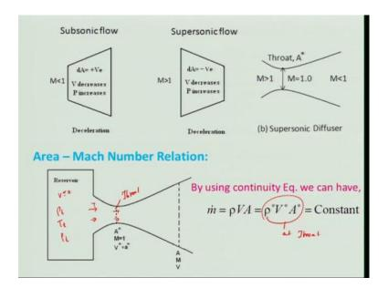
So, if you look at, this is basically the supersonic, diffuser where the flow is subsonic at the entrance and it goes out decreases, because the flow is supersonic and then it decreases further after passing through the throat. This is being used in your air intake kind of thing, which we will be discussing little later on, when you are discussing about cycle analysis.
