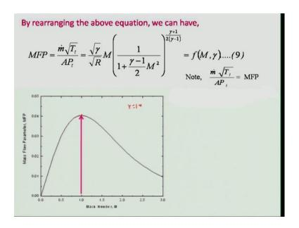
So, what you saying, this mass flux ratio will be function of P T, function of Mach number. Then, gamma which we will little bit simplify in the next and see that. So, by rearranging this, I can get this M dot root over t, A P T what I am calling it that mass flux
