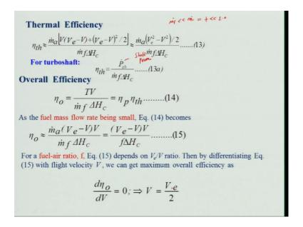
Now, we will be looking at thermal efficiency, because this is about propulsive efficiency which is tell you how good your engine is giving providing the what we called thrust
