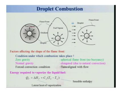
So, let us look at a three situation one is droplet is a spherical flame other is a droplet around that along get at flame, when there is a velocity if I look at these this is thing flame is coming that way. So, the three situations will occur that this will occur you know when the spherical flame, this is spherical flame and under zero gravity, that means, there is no gravitational effect or gravity is very 0, very small it tending toward 0 rather we have done some work.
