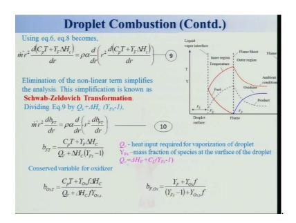
So, if I will do that then I can write down you know m dot r square d c p t plus y f delta s c divided by d r is equal to rho alpha, because in place of d I am putting alpha, because Lewis number is equal to 1. So, I can write down this term, now it has been simplified the none linear return as gone away in case of premixed flame, if you remember what we
