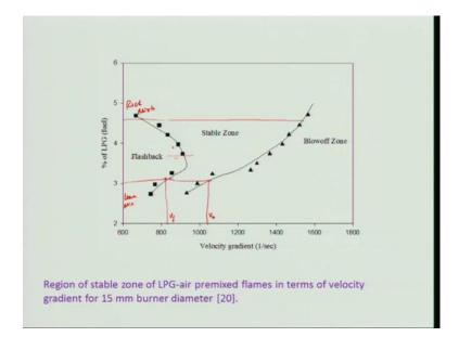
So, how it is occurring we will be looking at, I have taken a percentage of fuel in the y axis and x axis, I have taken velocity gradient 1 hour second. If you look at this d v by d r and you know meter per second it be can just 1 hour in 1 hour second or second in
