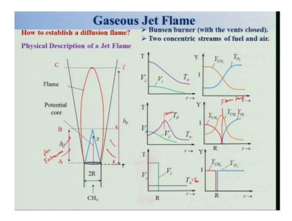
So and how to establish a diffusion flame or a rather a jet diffusion flame, which is a very simple like, we can use a Bunsen burner with a vented cloths. You remember that
