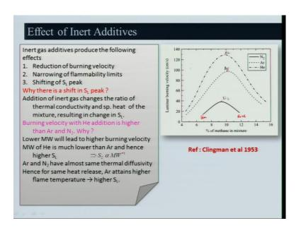
So, let us look at effect of inert additives like if I look at this the 3 additives one kind think of for a methane air flame and laminar burning velocities plotted with respect to the percentage of methane in the mixture. You can see that when it is nitrogen the burning velocity is very very low around 30 peak value is around 36 or 37 meter per second, but
