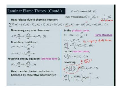
So, and what are the boundary condition if you look at of course, already talked about it T is equal to T u x minus infinity d T by d x 0, x positive infinity it will be t is equal to T F d T by d x 0. And as I told you we will be looking at this preheat zone in case of
