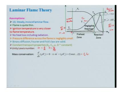
For the practical analysis proposes which will be doing keeping mind that this is our as I told you is a reaction the fuel flame and if I look at along with x direction when x is very far away. That means, x is infinity what will happened to temperature because temperature profile have shown here temperature gradient will be d t by d x will be 0 right yes or no and this is I am starting from here this is my origin.
