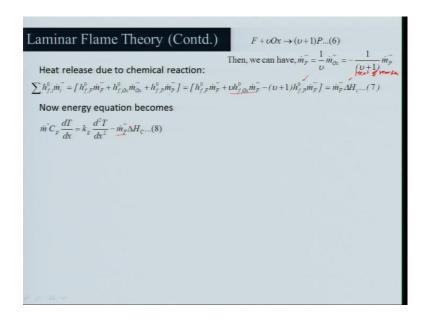
So, if you look at we are looking at this 1 K g of fuel reacting with nu K g of oxidizer going to the part of nu plus 1 K g of product. So, we can write down that m dot triple dash F, that is mass of fuel per unit volume being consumed is equal to 1 over nu m dot triple dash O x is equal to minus 1 over nu plus 1 m dot triple dash P. why it minus because this fuel and oxidizer is being consumed whereas, product is being formed instead of righting minus here I have put here.
