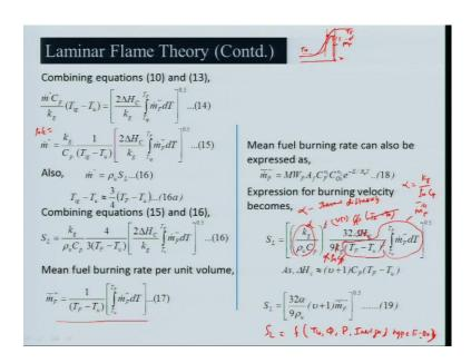
So, combining this equation ten and thirteen we are getting m dot double dash C p by K g T i g minus T u equal to route over 2 delta H c K g integrated over m dot triple F d T it is integrated over T ignition to T F. So, if you look at still we are not solving because we need to integrated this you know integration that it is not really possible because you do not know that temperature, how it is varying with temperature and the T ignition is also not known.
