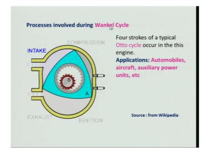
So, I will be discussing about wankel engine I am very much fascinated by this engine, because it is quiet compact, it works on a basically four stroke of a typical auto cycle in this engine, you can look at in this animation that air is coming over this known as air intake it will be compress, and then once it compress then the ignition the combustion take place over here, and then it will be expanded and it will be going to the adjust.
