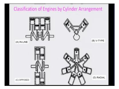
Based on the cylinder and piston arrangement we can classify the engines into four, but of course, you can have more, but here as shown the four type, one is inline engine, if you can look at there are several piston cylinders are connected to a same crank shaft, but with different phases phase angles such that it can move randomly or move in a continuous manner without much fluctuation in the power label on the load on the crank shaft.
