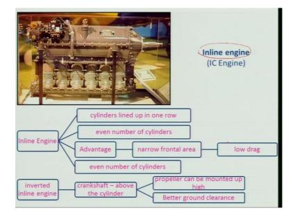
So, under this category I will show you two engines, one is inline engine as I told that it is being use by the right brothers, and which is having a cylinder these are the cylinders, which is lined up in one row, and if you look at generally piston on the top, but here in this case pistons are in the bottom and this is the crank shaft, which is having a shaft.
