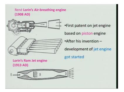
And of course, the air breathing engine concept was given by a genius I call it Rene Lorin and who gave a concept taking from the piston engine I will show you a figure here, and in this case this engine is basically connected with a with a nozzle, which is you can call it as convergent divergent nozzle, and this is the cross sectional view.
