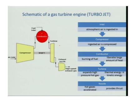
So, if we look at as shown this schematic diagram here, there I have showed you a cross sectional view, which is air will be entering into compressor and this is the combustion chamber, and the turbine keep in mind. The turbine will be producing power, which is just mean to run the compression it would not be giving you any thrust and of course, the thrust will be obtain by the by expanding the gas in the exhaust nozzle. So, that is a basically what you call the turbo jet engine.
