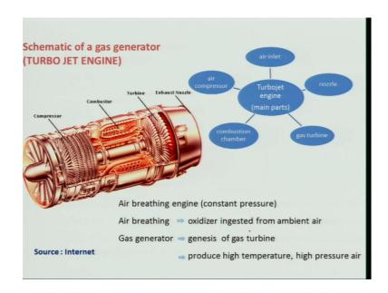
So, let us look at a gas turbine engine that basically it is a gas generator, which has shown here, this having a compression is having a combustion chamber, and this is having a turbine, and this constitute the gas generators and whenever the gas generator is connected with a nozzle and at air intake, which is not shown in this figure is consider as an aero gas turbine engine or turbo jet engine right.
