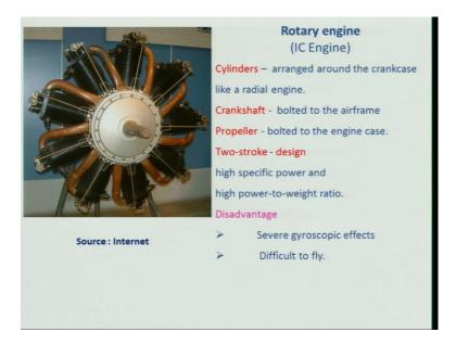
And of course, there are several re-engines, which is together having use and there is another engine which you can see in our flight lab, which is being kept as a model I guess it is a rotary engine; that means, the cylinder these are the cylinders, which are being mounted along with the thing and as result it will be well balance right.
