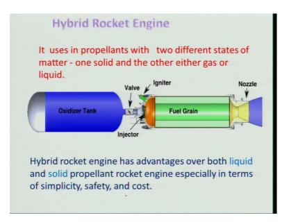
So, let us look at a hybrid engine, where the both solid fuel like grain is being use and oxidizer, and it is having abuse, because it is having several advantages over both the solid and the liquid propellant engines. So, either one solid or are even the gas or the liquid can be combine to it.
